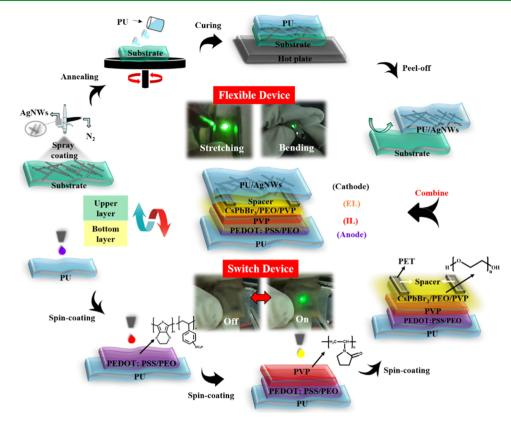
Figure 1. Schematic of the fabrication process of stretchable LETD. Photographs of stretchable LED and LETD under 5 V.
